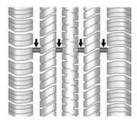
One way to tell when it is time for new tires is to check the treadwear indicators, which appear when the tires have only 1.6 mm (1/16 in) or less of tread remaining. See *Tire Inspection on page 10-72* and *Tire Rotation on page 10-72* for additional information.
